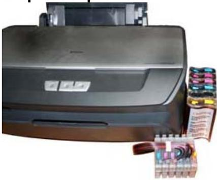
Put the CISS on the right side of the printer. and place all the tubes at correct position.
