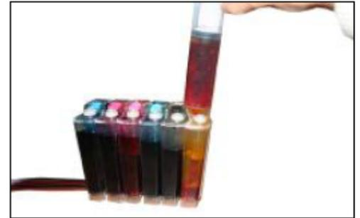
Please pay attention to the ink level in the reservoirs; if the ink level is below 1CM as the picture shown above, please use refill kits to fill ink into Reservoir bottles. Carefully pull out the rubber plugs from the ink refill holes (There is a possibility of ink spattering. Please be careful.) Refill ink according to the colors. Then re-cap the rubber. **(Please keep the printer and the reservoir bottles at the same level while refilling ink.)**
