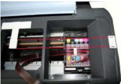
Stick the clip on the right side of the printer, make sure the tube and the printer are in between the parallel line.
