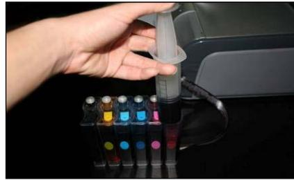
***\*Note: During the refill process, please keep the reservoirs and the printer horizontally aligned on the same surface.***
