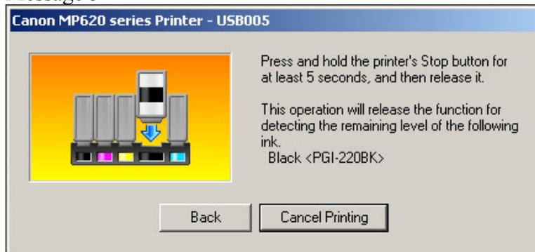
Press and hold the printer's STOP button for at least 5 seconds, and then release it.
