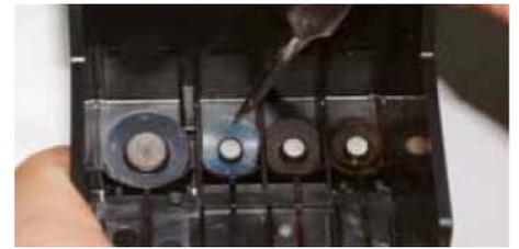
Carefully place each silicon nozzle seal into position around each of the printer heads as shown. Make sure that seals do not move from position when inserting cartridges. These seals must not be interfering with the silver print head. Incorrectly placed seal can cause poor ink quality.
