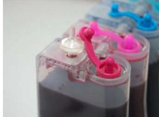
Place air filters into air holes, For all colors. With the fat side down
