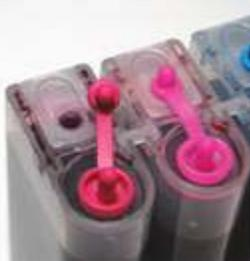
Pull out the small rubber plug from the air hole as picture shown above. For all colors
