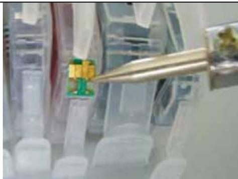
Place the chip onto the CISS cartridge ensuring that the small plastic lugs are inserting into the chip holes. You can melt lugs with a soldering iron (or anything that's hot) or glue the chip in place (do not use super glue because it will damage the chip). If using a soldering iron gently melt the plastic lugs to hold the chip in place.
