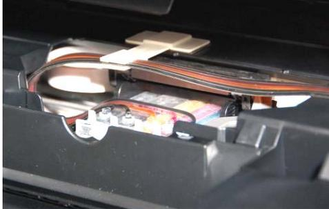
Install ink line holding T clip and the ink line as shown in the picture.
