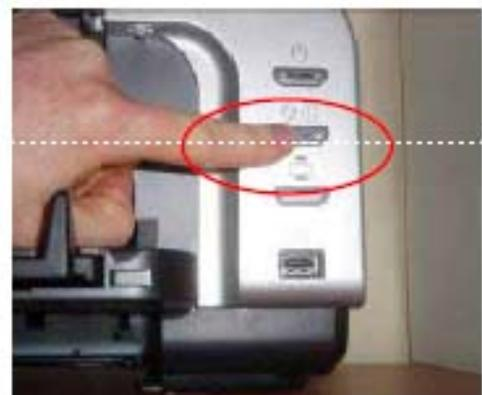
You do not need to remove or replace the cartridge when this message appears. Simply press the printer resume button followed by OK.
