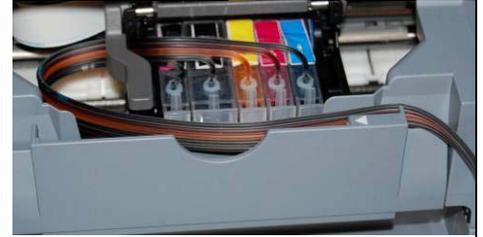
Unplug the printer again. Install the ink line as shown above. Make sure ink line is not twisted. Make sure printer is unplugged before moving print head left of right
