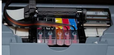
Install print head and install Cartridges in the printer. Plug Printer in and Make sure all of the cartridges light up. If any are not lit up that means chip on that cartridge is damaged or not installed correctly. Printer won't work until all cartridges are lit up.
