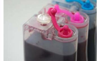
Place air filters into air holes,
