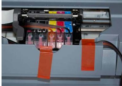
Install two pieces of tape to hold the ink line in place. You can use any good invisible tape. We used orange tape so that it will show in the picture.
