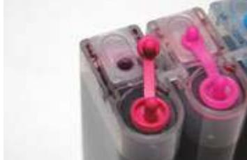
Pull out the small rubber plug from the air hole as picture shown above.
