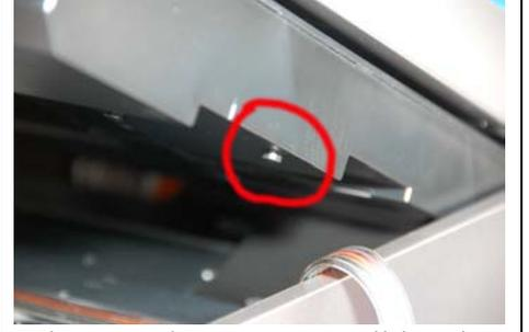
When you lower scanner lid make sure scanner leg does not land on the ink line.
