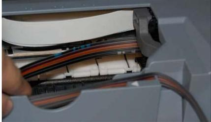
Hold ink line with your finger and move the print head to the leftmost and rightmost to make sure that there is enough ink line to reach both ends.
