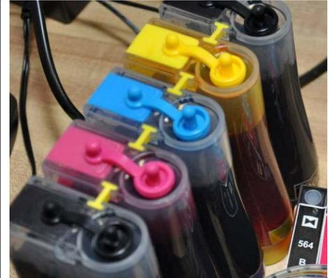
Make sure ink tanks are sealed for the next step of the install.
