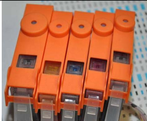
After you are done installing the chips make sure to put orange ink cover back on. **Never leave CISS cartridges for long periods of time with covers missing. Ink will leak from the cartridges.**
