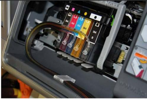
Install ink line clip in the middle of the printer to hold ink line in place. As shown in the picture above.
