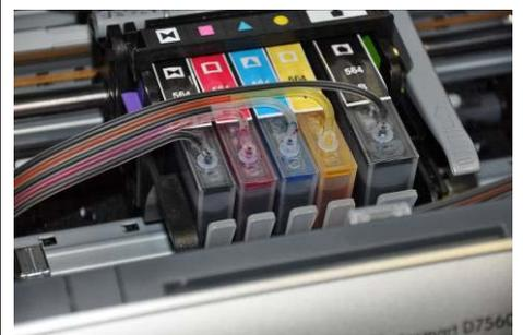
Properly install cis cartridges. You may see some air in the ink tubes however do not be alarmed It is normal to have some during initial install. Only if the cartridges are all the way empty you will have to refill them.(Refill instructions are on the last page at the end.)
