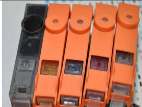
Remove orange ink cover corresponding to the color chip you have removed.
