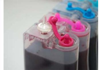
Place air filters into air holes, For all colors. With the fat side down
