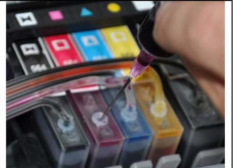
Use syringe with a needle and refill cartridge as needed. Do not overfill or the ink will leak out of the top. Reconnect ink line. Rinse syringe with water for next use.
