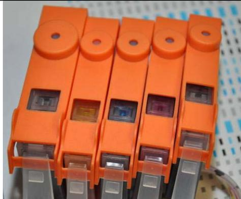
Place cartridges upside down and have a paper towel handy in case ink leaks from the cartridges.
