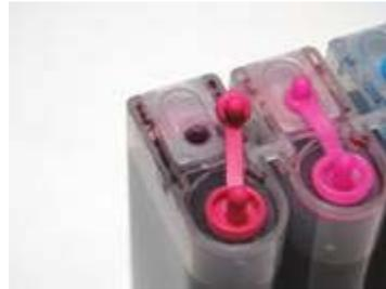
Pull out the small rubber plug from the air hole as picture shown above. For all colors
