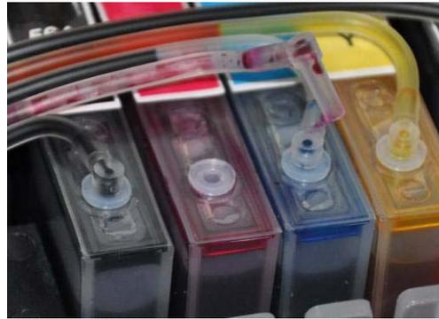
Disconnect ink line from the cartridge. By pulling it out
