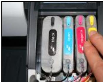
Slightly press every cartridges to check all the cartridges are in the correct position.
