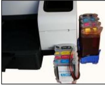
Put the CISS on the right side of the printer, in the same time order all the tubes in the correct position.
