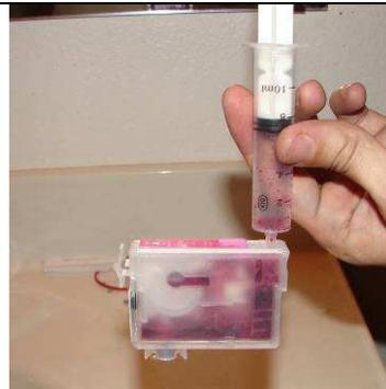
Simply let go of the handle and the vacuum you created will draw the ink into the cartridge. If there is any ink left in the syringe pull back to 10ml and repeat the vacuum step again. Again **DO NOT PRESS DOWN ON THE HANDLE OR TRY TO INJECT THE INK!**
