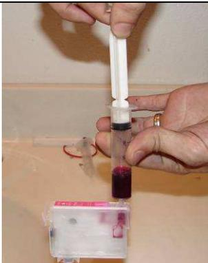
Do not press down do not try to inject ink. Instead, hold syringe with one hand pull handle up until it reads at 10ml. This draws the air out of the cartridge and creates a vacuum.
