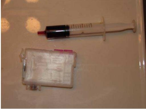
Fill syringe with 4ml of the correct color of ink needed
