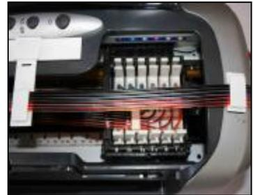
The tube is excessive long, it is not ok. The tube is twist ,it is not ok. In this situation ,it is ok
