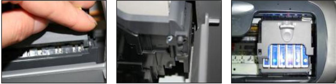
Then press the right side of the cartridge cover to make it down to the suitable position, now it is ok to work.
