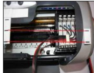
Fix the balance arm stick on the support arm as show on the picture, Rip the label on the shortest arm ,And Stick it on the right side of the printer, but need to keep it in the same horizontal line as show in the picture
