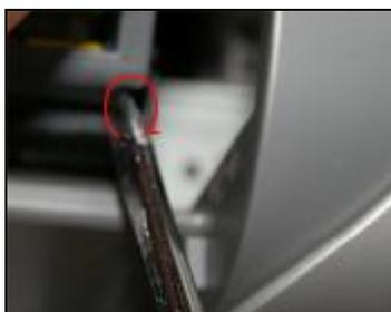
And screw the screwdriver in clockwise till the right side of the cover divide from the connection on the cart, then take down the cartridge cover
