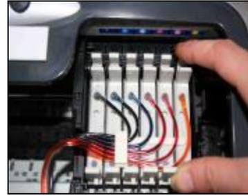
Remove out the original cartridges ,then place down each cartridge according to the color ,in the meantime, make every cartridge in the correct position.
