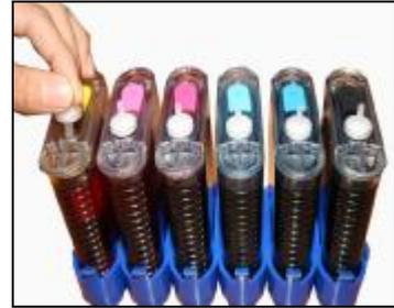
Place 6pcs of air filters into air holes, the thicker side is down into tank.
