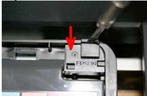
Insert the screwdriver into the slit, push it down slowly. And remove the clip
