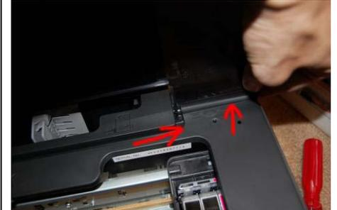
Pull to the left and then up to remove printer cover.
