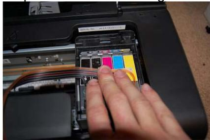
Install Cartridges make sure push down firmly. Make sure you hear a click for every cartridge.
