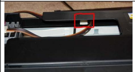
Attach ink line clip inside the printer like shown in the picture. Make sure to press firmly. Or glue it with super glue to make sure it does not come loose.
