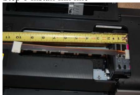
Measure 10" from the cartridges and install ink line clip on the ink line.
