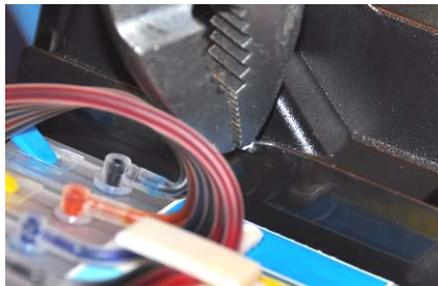
This will allow for the ink to flow freely into your printer. 1) This printer will not work if the lid is open even just an inch. 2) The ink lines will get pinched preventing ink from flowing into your printer.
