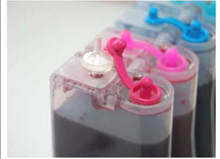
Place 6pcs of air filters into air holes, For all 6 colors. With the fat side down
