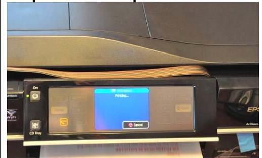
You are almost done! Make sure there are no sharp edges in the plastic that will cut the ink line. Push printer lid carefully down until printer says that it is down.
