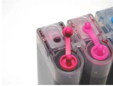
Pull out the small rubber plug from the air hole as picture shown above. For all 6 colors
