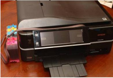
Put the CISS on the Left side of the printer. and place all the tubes at correct position.
